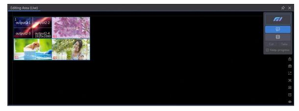
• The sequence number in the upper left corner of the slice indicates the layer slice in program management. This number corresponds one-to-one with the layer number, which can be modified in the **Bind Input** section of the properties.
